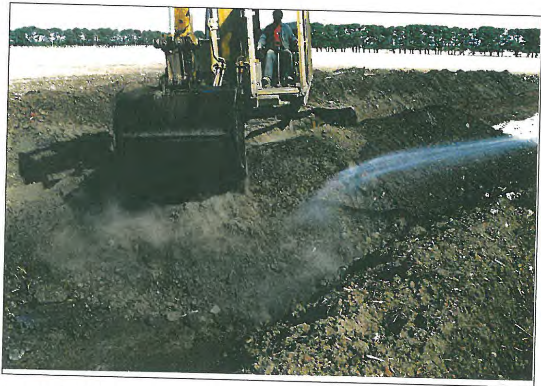
Figure 4. The mixing process during the formation of the windrows
