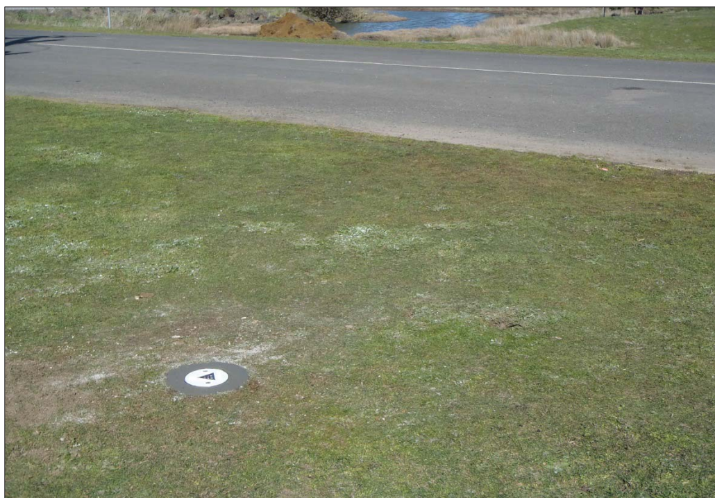
Figure 4-3: Protective Cover on Bore GW107
