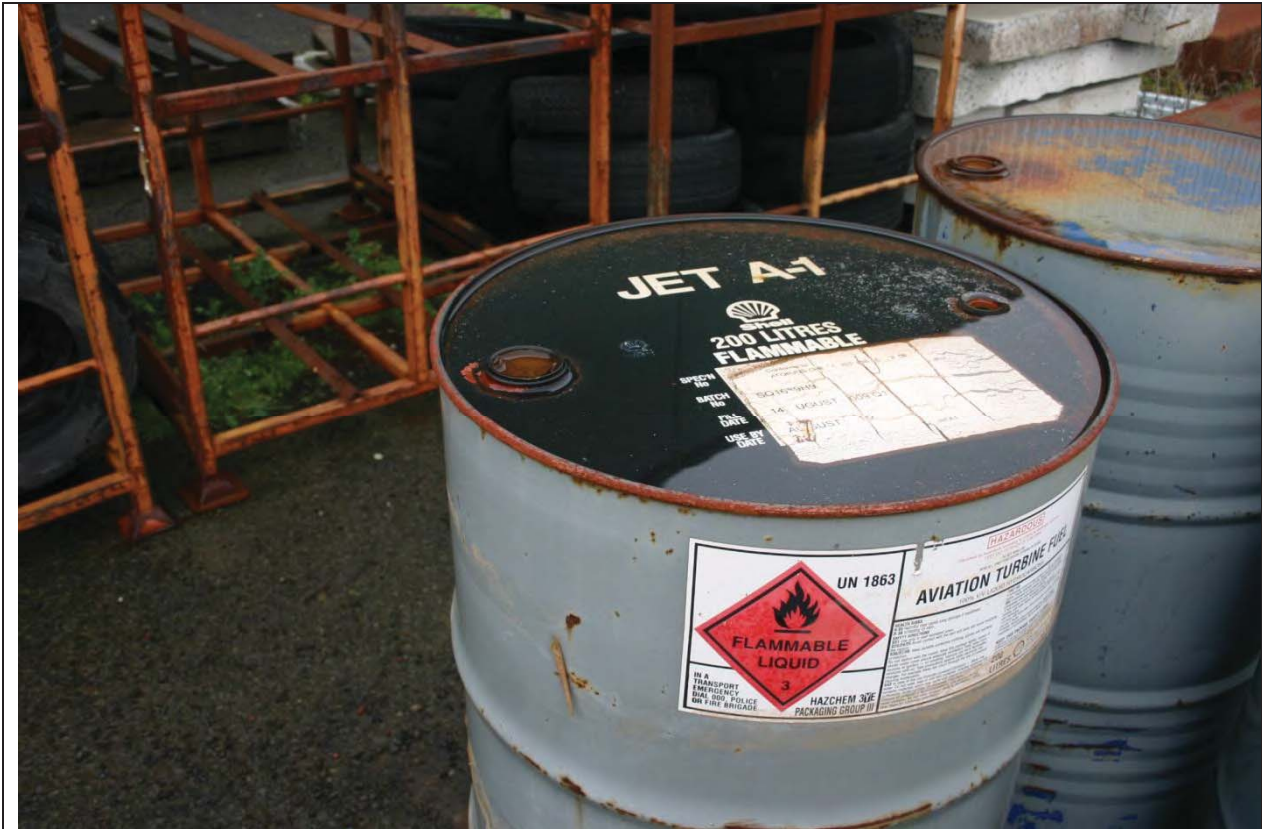
PLATE 11 Drums containing Jet fuel - Unbunded (13 July 2013)
