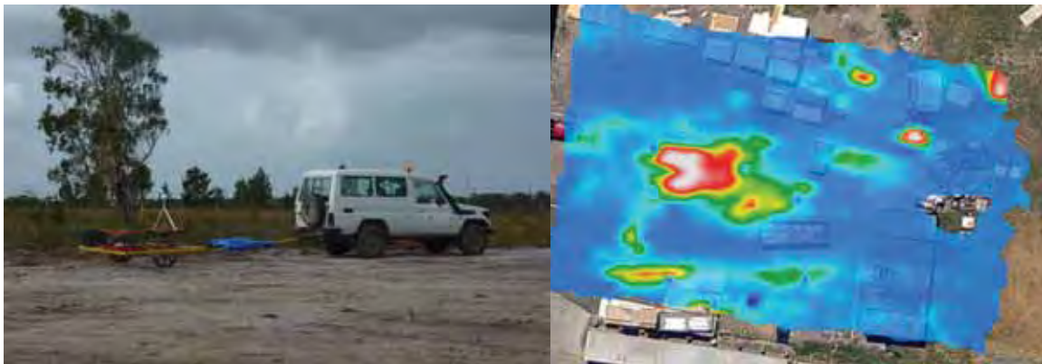
Figures. A) Collecting TEM data with the EM61 and B) Sample of processed data.
