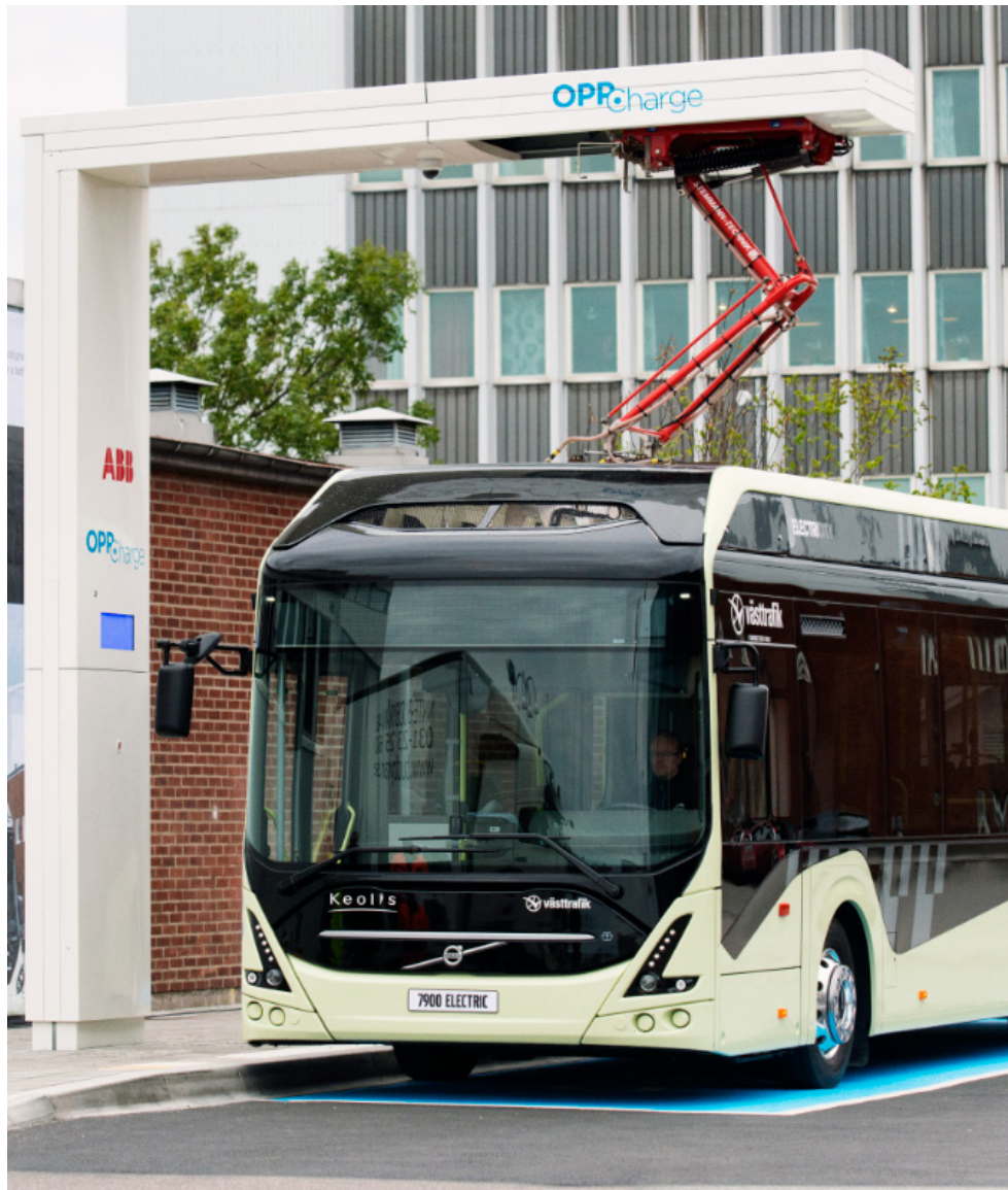
Figure 4.4 An electric bus recharging from an inverted pantograph, in front of Volvo in Gothenburg, Sweden, from the global ABB website
