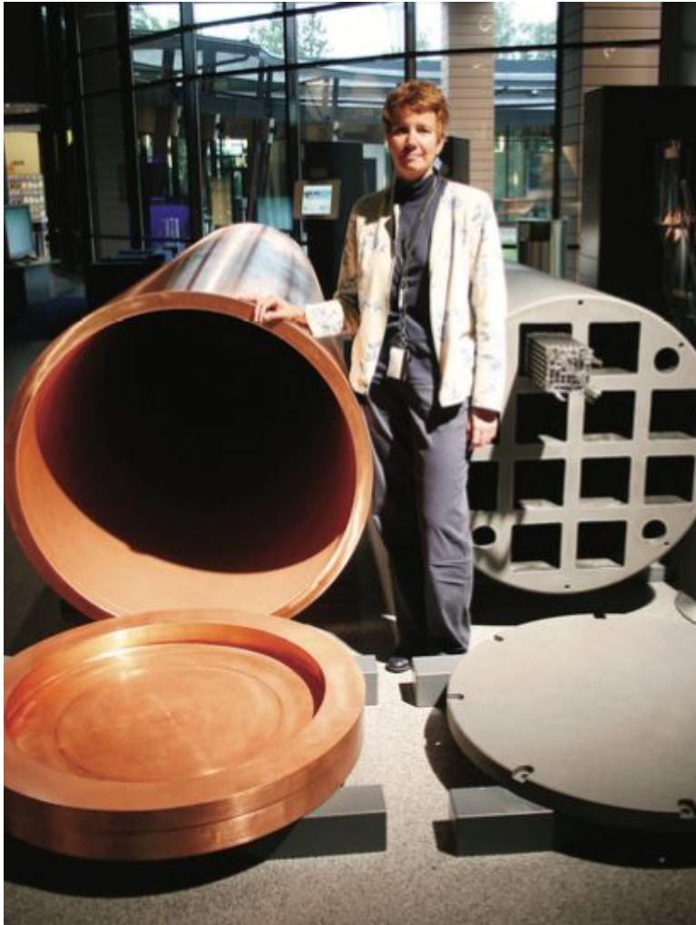
Copper and iron components of the 26 tonne waste storage canisters from Finland's Onkalo nuclear waste storage facility — an example of downstream material usage, omitted from the materials analysis. (Photo: Sandra Upson. Source: IEEE.org )
