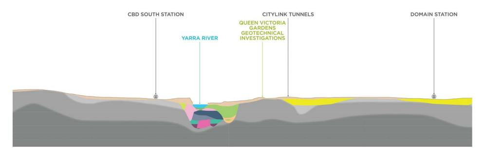
Previous work shows there are a variety of different types of materials under the river including basalts, silts and clay.
