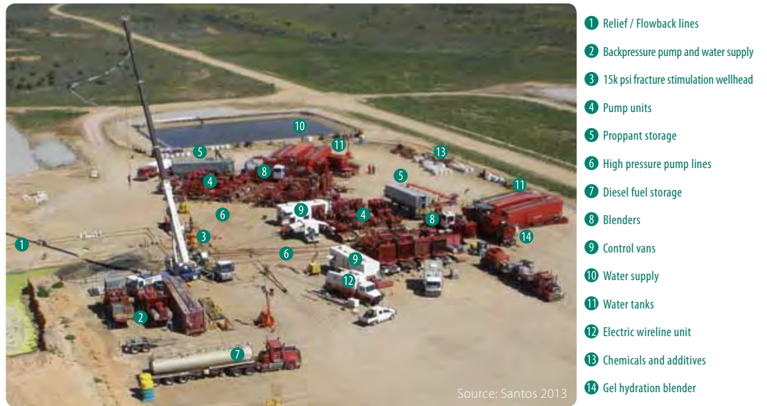
Figure 4.3 Well stimulation by hydraulic fracturing in Australia
