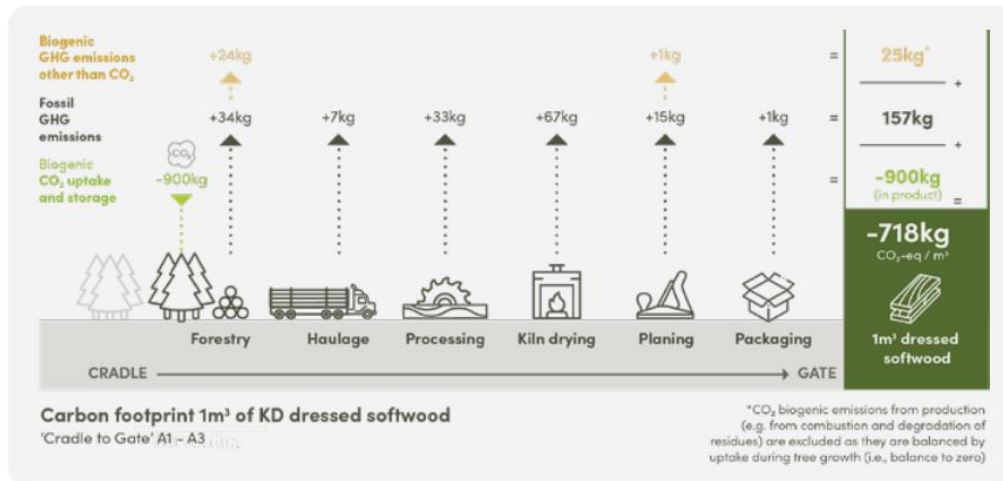
Figure 5 - Carbon footprint of 1m 3 of kiln-dried dressed softwood (FWPA, Australian Sawn Softwood EPD S-P-00560 v2.0, 2022)
