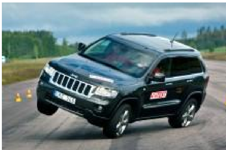
Figure 31 Tekniken Varld Jeep Cherokee "Moose Test" at 63.5km/h in 2012
