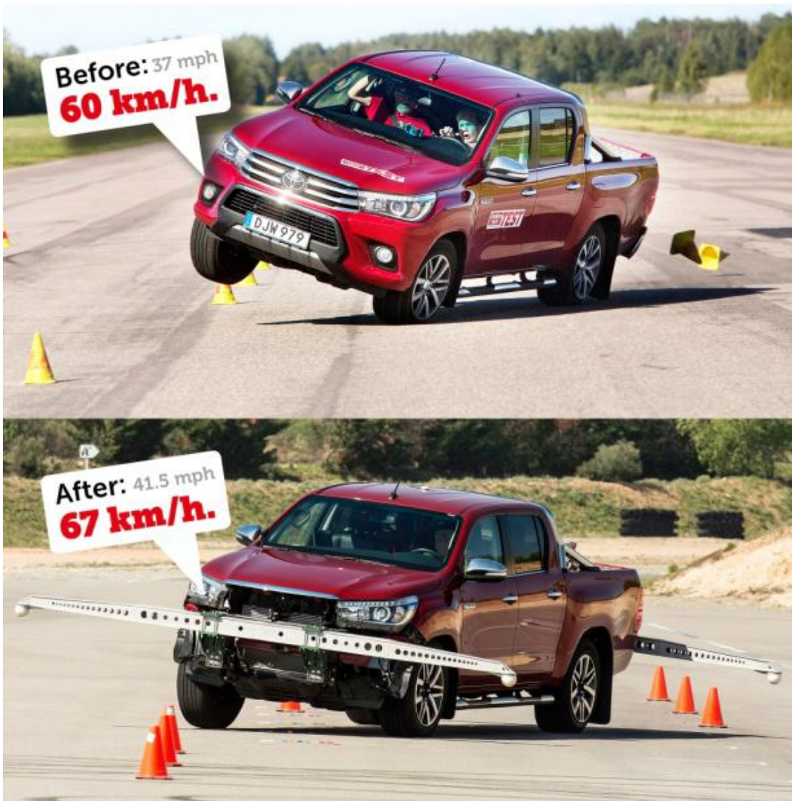
Figure 29 Toyota Hilux initially failed the "Moose Test" - then redesign and modified in 2017
