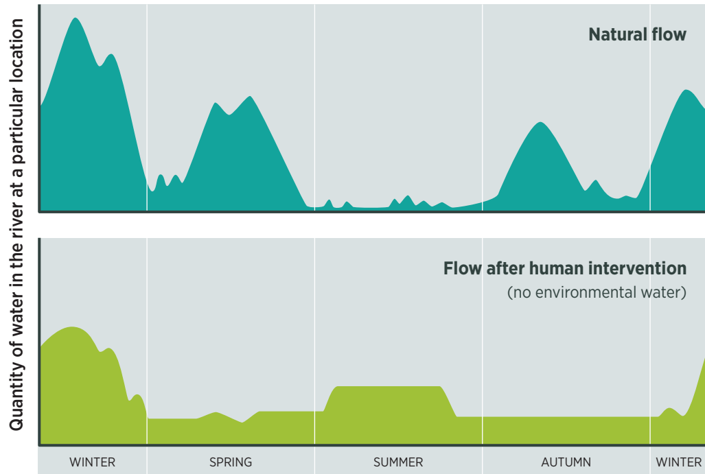
Source: Environment, Natural Resources and Regional Development Committee, adapted from Victorian Environmental Water Holder in Victorian Government, Submission 39 , Appendix 2, p.11
