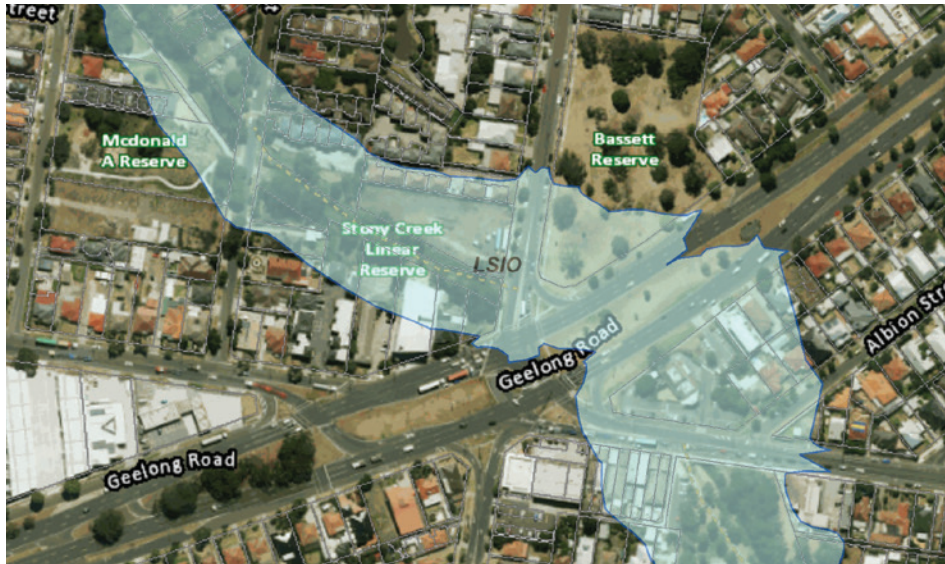
Figure 4.8 A land subject to inundation overlay (LSIO) in the Maribyrnong Planning Scheme
