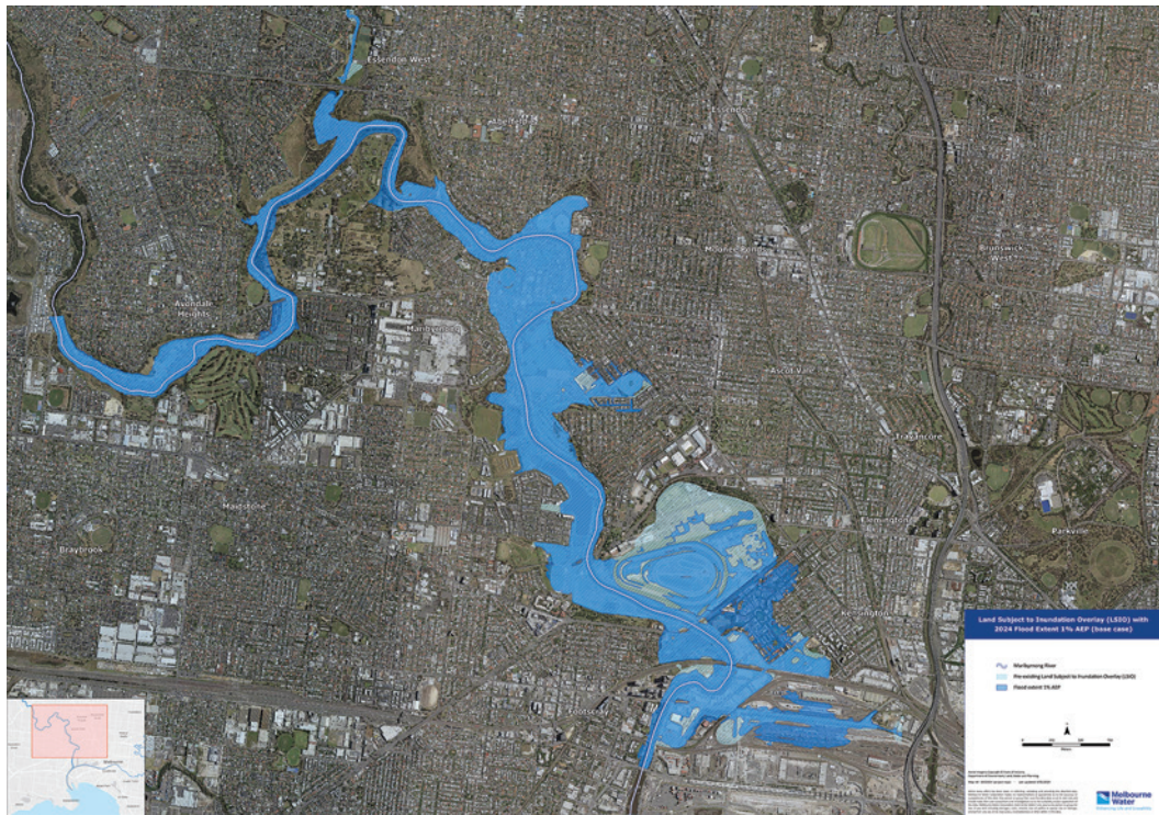
Figure 4.12 Comparison between the 2024 Maribyrnong River 1% AEP flood extent and the pre-existing land subject to inundation overlay
