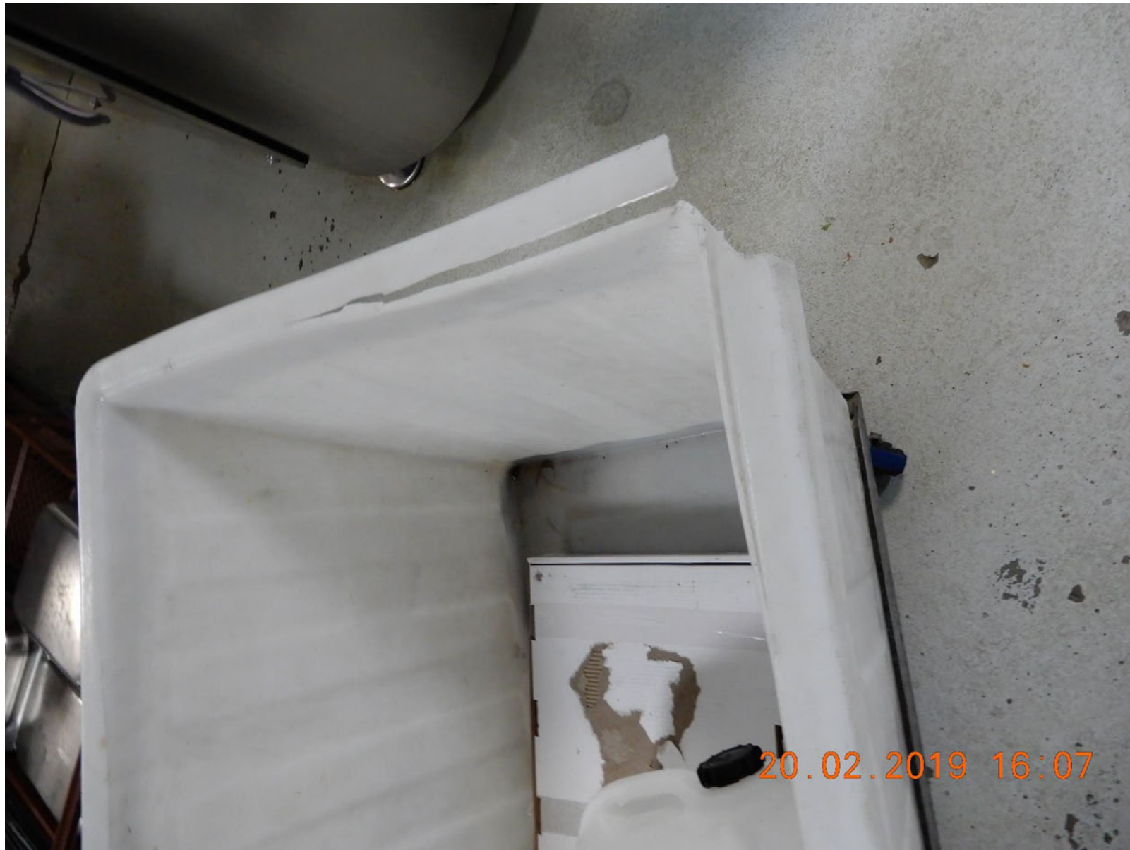
EG270: Photograph of broken and damaged tub on a trolley being used within the Main Food Preparation Area.
